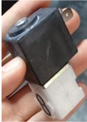
Gambar 2. Komponen Valve Two Way
