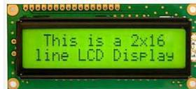
**Gambar 4. LCD (Liquid Crystal Display) 16x2**
