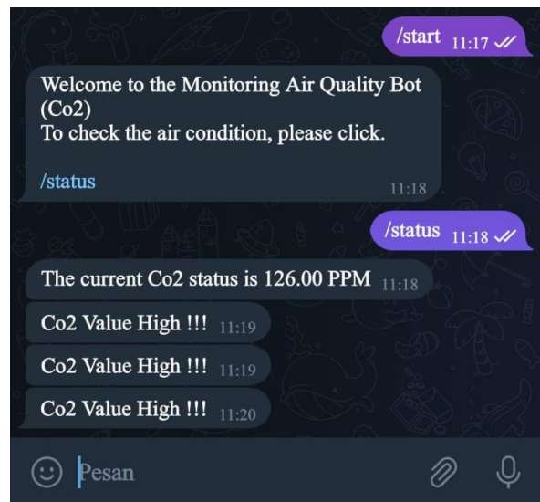
Figure 10. If the CO2 gas value is harmful, then the Telegram bot will notify users with the message "Co2 Value High !!!! "
