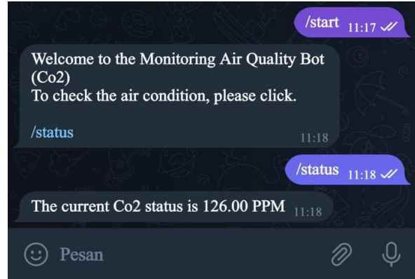
Figure 9. Click status to find out the amount of CO2 gas present in the room; the value will then be displayed.
