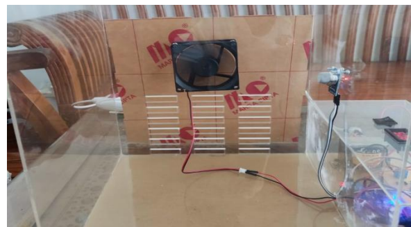
Figure 11. The fan will automatically activate to remove CO2 gas from the room.
