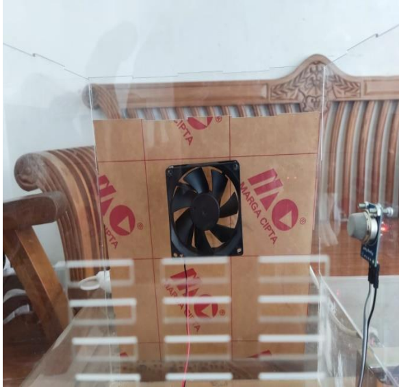
Figure 12. After the CO 2 level has decreased to a predetermined value, the fan will stop.
