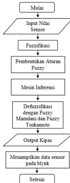
**Gambar 1. Alur Proses Sistem Kendali *Exhaust Fan***
