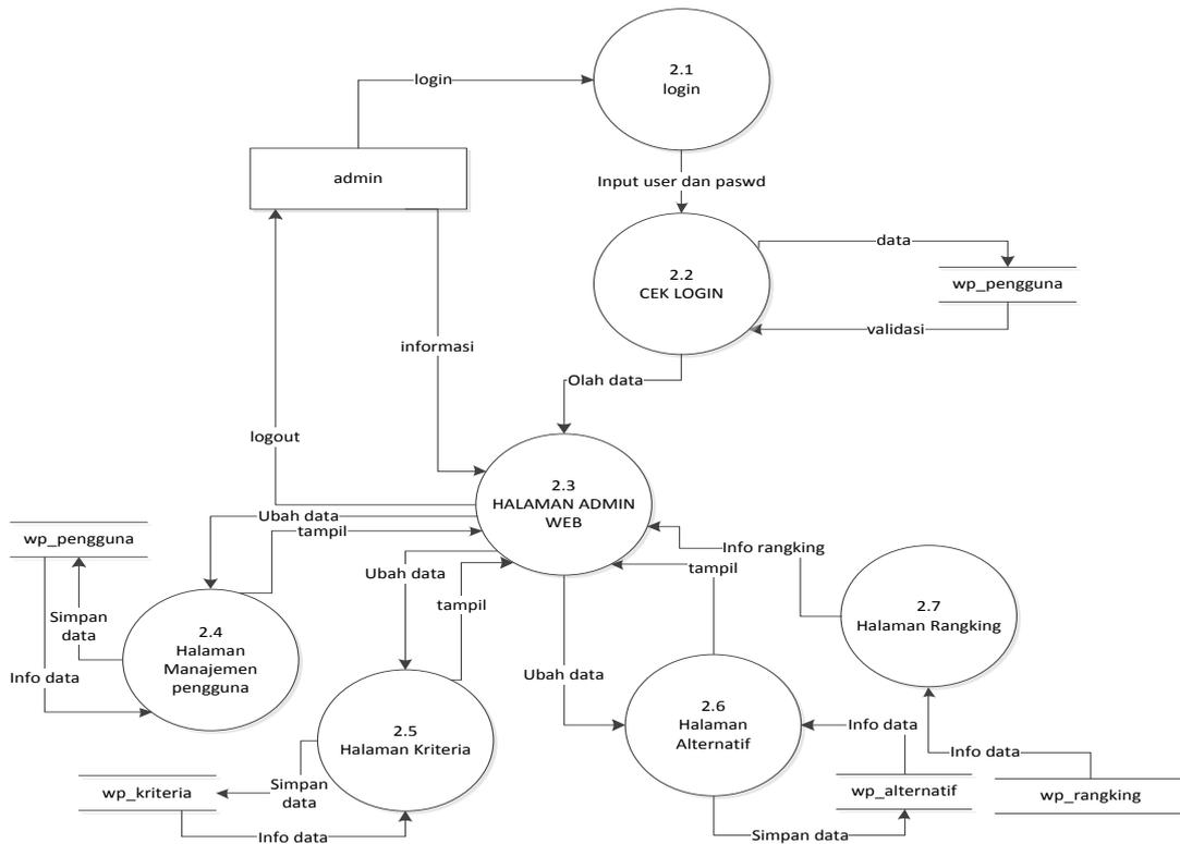
Figure 3. Data Flow Diagram level 1 Process 1 and Process 2
