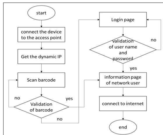
Fig 13. Flow of using smart wifi
